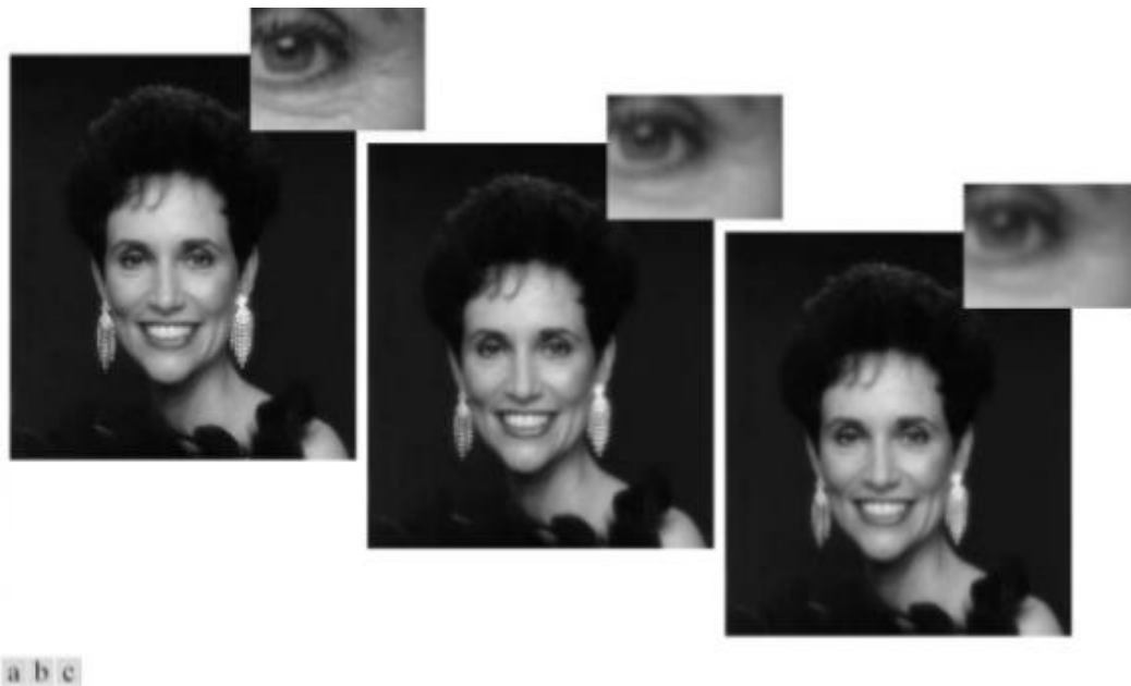
Fig. (a) Original image (784x 732 pixels). (b) Result of filtering using a GLPF with D_0 = 100 . (c) Result of filtering using a GLPF with D_0 = 80 . Note the reduction in fine skin lines in the magnified sections in (b) and (c).
